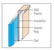
**Cool Technology** Insulated walls feature SEALED gel packs for optimal cold
